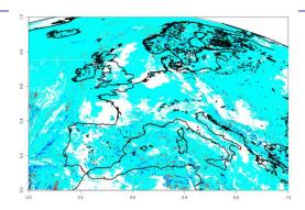
Latest addition in the expanding portfolio: ctth\_effective (defined as fraction of the field of view covered by clouds (cloud amount) multiplied by the cloud emissivity in the 10.8 μm window channel).
