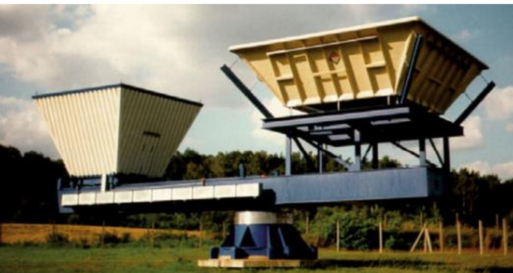
1290 MHz boundary layer wind profile radar (RASS LAP 3000)
