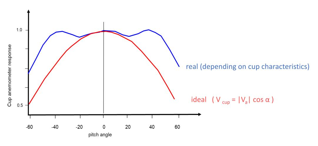
→ Overestimation different for each sensor, align sensor horizontally; slopes ?
