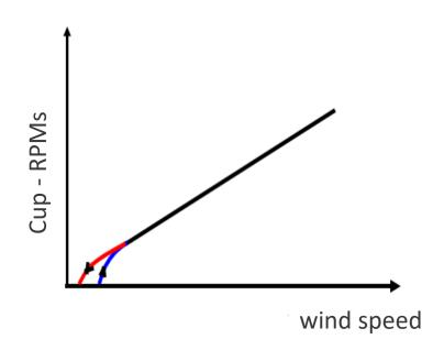
$\rightarrow$  Overstimation depends on: cup characteristics (mass, shape, dimensions) speed and gust characteristics
