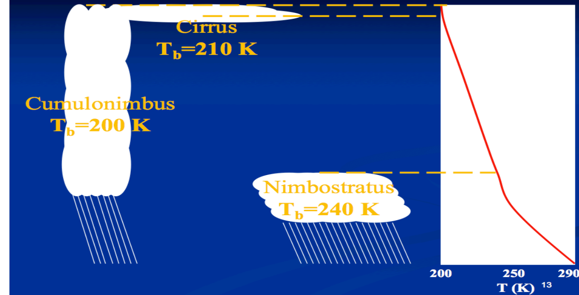
Illustration of the IR signal from different cloud types
