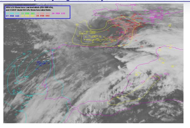
Comparing against ECMWF Model wind fields, HRW confirms the NWP model forecast (trajectory of Xynthia and the areas suffering the strongest winds), although in general winds are weaker than expected.
