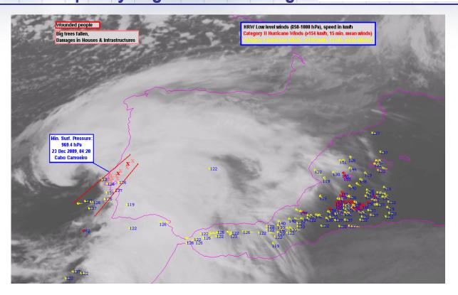
HRW product identifies a narrow area of Hurricane force low level winds coming from the ocean in the area where the main damages occurred (15 min. mean winds between 125-150 km/h in the layer 850-1000 hPa)
