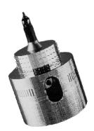
Nimbus 7: THIR – Temperature-Humidity Infrared Radiometer
